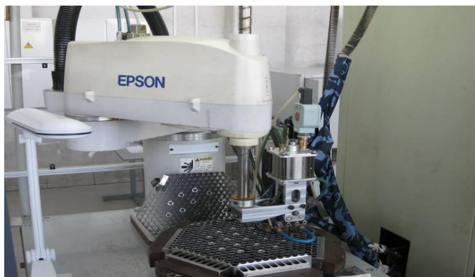
Robotized complex for spot welding of spacer grids
