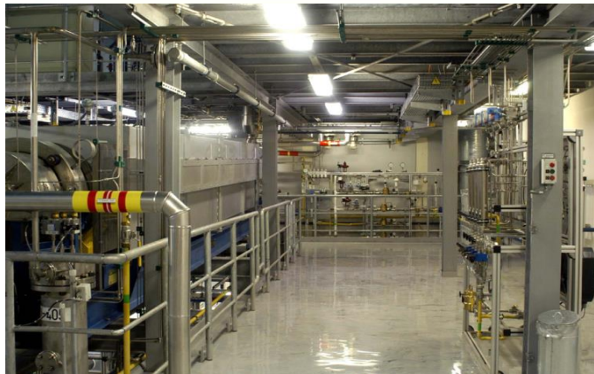
Section for producing uranium dioxide powder by "dry" conversion technology
