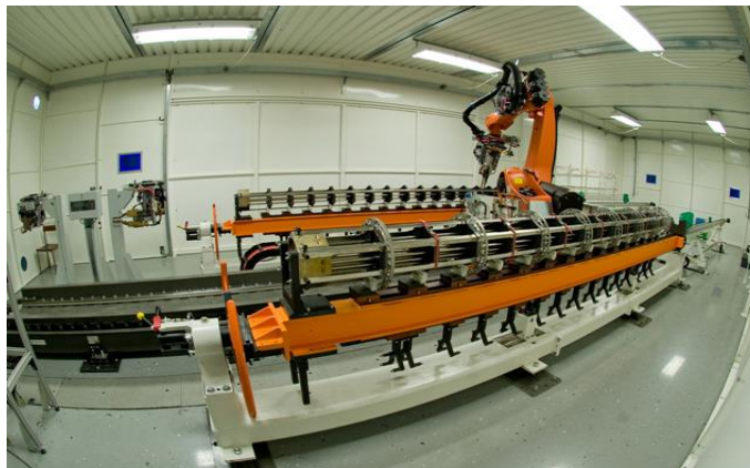
Robotized complex for assembly and welding of FA skeletons
