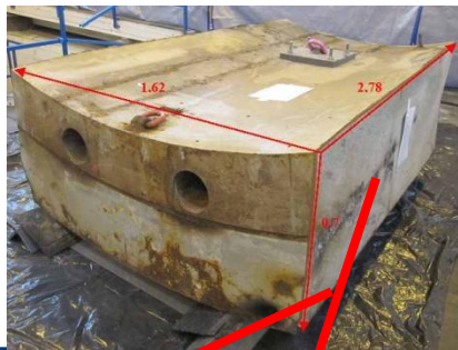
Part of the reactor biological shielding from NPP Greifswald
